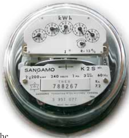
Figure 9.17 The electricity meter in your home may be similar to this one. The middle disk turns, showing the rate at which electrical energy is being used within the home.
