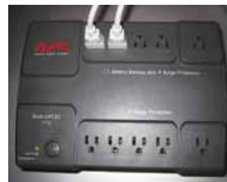
Figure 9.18 An electrical surge protector
