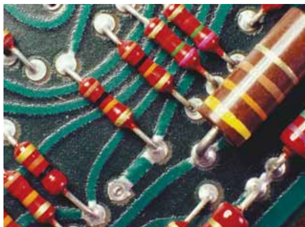
Figure 8.19 Resistors are used to control current and voltage in electrical circuits.
