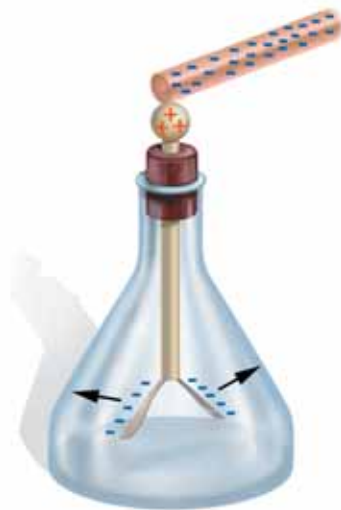
Figure 7.11 A negatively charged rod adds extra electrons to the electroscope.
