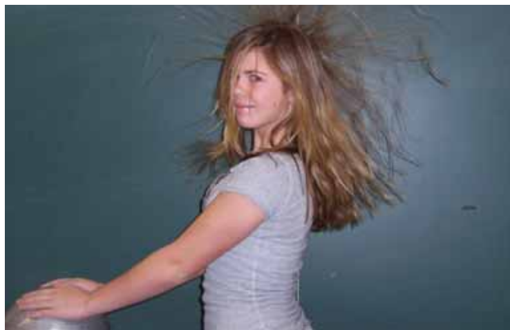
Figure 7.6 A Van de Graaff generator produces enough static charge to give a student a “hair raising” experience.
