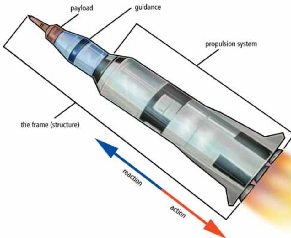
**Figure 12.26** All rockets have four main systems: structural (the frame), payload, guidance, and propulsion. The payload is the cargo that the rocket carries. It could be astronauts, satellites, or other objects. The propulsion system produces thrust, the force needed to launch the rocket.
