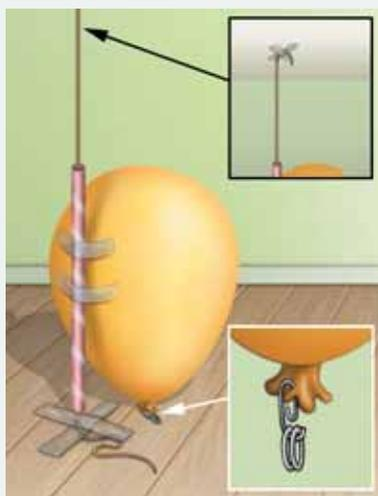
In this activity, you will simulate the forces needed to generate thrust in a rocket engine, and you will determine the maximum thrust of a balloon rocket engine.
