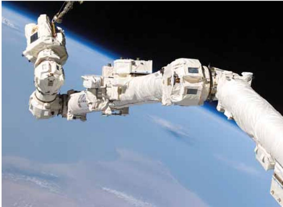
**Figure 12.30** Canadarm 2 is used to move large payloads, dock the shuttle, and assist astronauts with repair and assembly duties.
