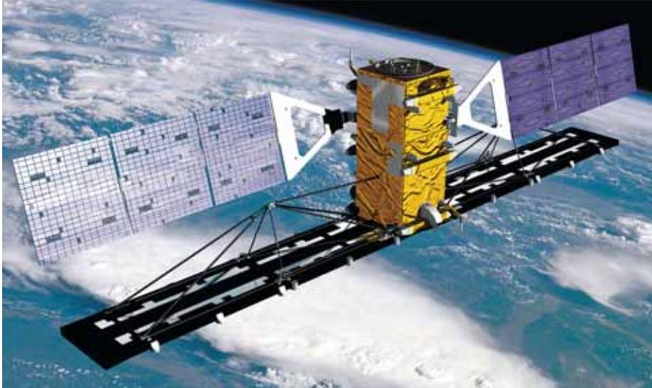
**Figure 12.23** *RADARSAT 2* orbits at an altitude of 798 km and has many uses, such as geological mapping, forest mapping, iceberg detection, and marine surveillance.
