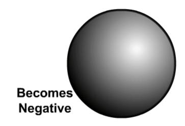
Electrons transfer to the object making it the same charge
