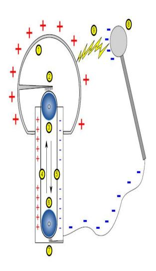
A Van de Graaff generator uses friction to produce a large static charge on a metal dome. The moving belt produces a static charge at the base, and this is carried to the top of the dome where it is collected.
