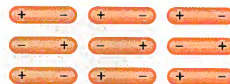
Figure 11.1 Molecules that have a permanent dipole moment tend to align with opposite polarities in the solid phase for maximum attractive interaction.
