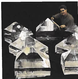
These giant potassium dihydrogen phosphate crystals were grown in the laboratory. The largest one weighs 701 lb!
