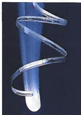
When magnesium burns in air, it forms both magnesium oxide and magnesium nitride.
