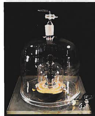
Figure 1.9 The prototype kilogram is made of a platinum-iridium alloy. It is kept in a vault at the International Bureau of Weights and Measures in Sèvres, France.
