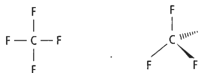
Figure 9B-1 Structural Formulas for \text{CF}_4 (a) two-dimensional (b) three-dimensional
