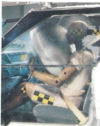
An air bag can protect the driver in an automobile collision.
