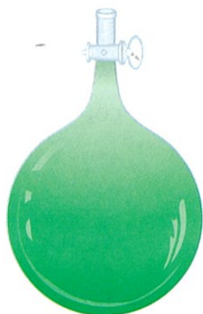
Figure 5.12 An apparatus for measuring the density of a gas. A bulb of known volume is filled with the gas under study at a certain temperature and pressure. First the bulb is weighed, and then it is emptied (evacuated) and weighed again. The difference in masses gives the mass of the gas. Knowing the volume of the bulb, we can calculate the density of the gas. Under atmospheric conditions, 100 mL of air weigh about 0.12 g, an easily measured quantity.
