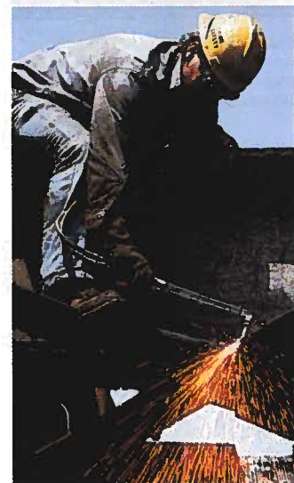
An oxyacetylene torch has a high flame temperature ( 3000^\circ\text{C} ) and is used to weld metals.
