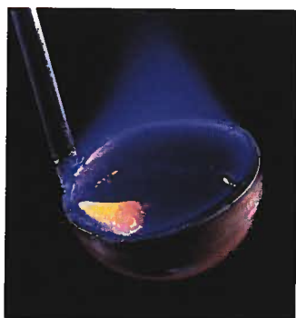
Sulfur burning in air to form \text{SO}_2 .
